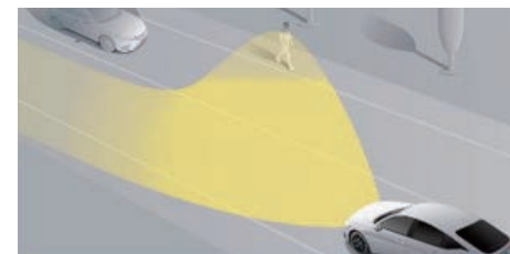
Adaptive driving beam system
