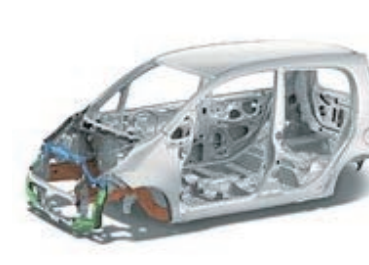
Advanced Compatibility Engineering (ACE) body structure
