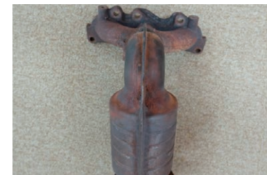
Cracked exhaust manifold of Honda Life mini-vehicle made in 1999
