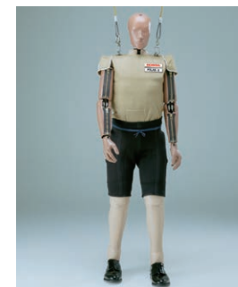
POLAR III, the third-generation pedestrian dummy
