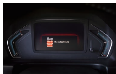
Rear Seat Reminder system and Rear Seat Camera system
