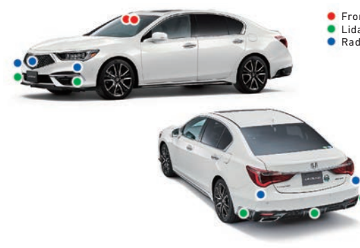
Layout of sensors of the Honda Sensing Elite
