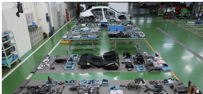
Verification of parts following durability testing
