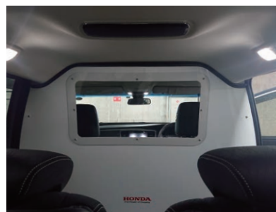
Interior of a vehicle used to transport COVID-19 patients (with a plastic barrier between the driver and rear seats)
