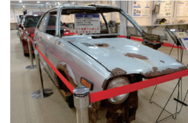
Rust on the body of a Honda Civic made in 1981
