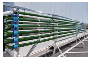
A close-up view of the algal farm, which collects CO 2 from a test dynamometer at HRA
