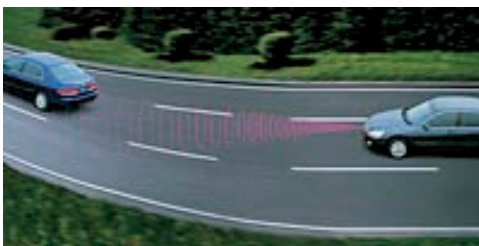
IHCC with Vehicle Speed and Inter-Vehicle Distance Control Functions
