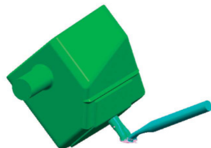
Fig. 7 Simulation model of in-cylinder gas motion
