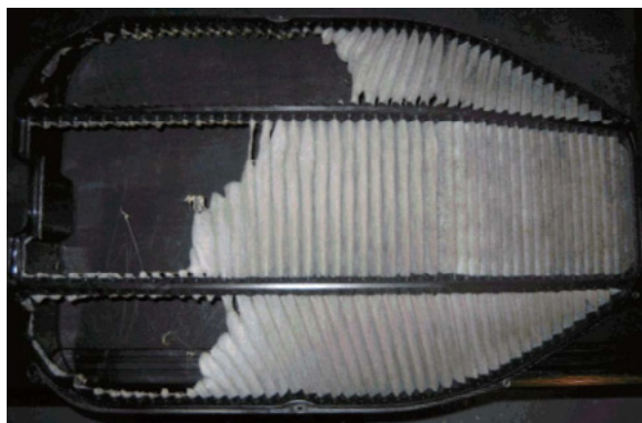
Fig. 2 Damaged air filter
