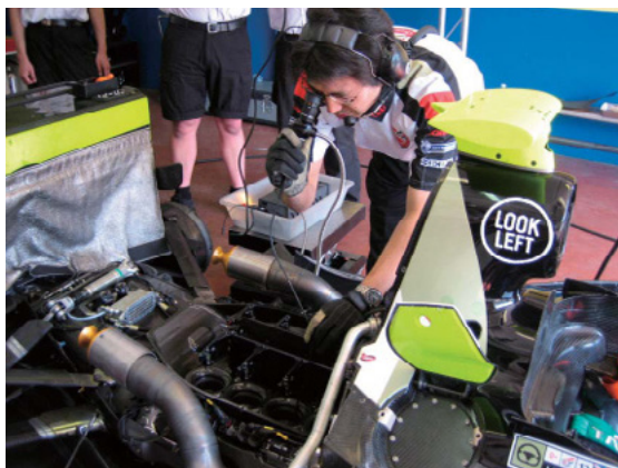
Fig. 4 Checking inside of engine
