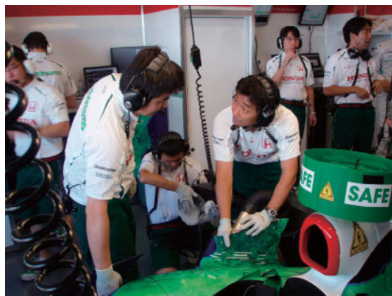
Fig. 5 Checking KERS system
