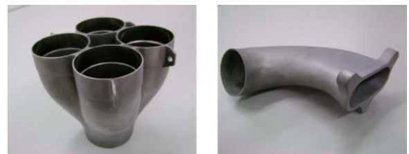
Fig. 7 Casting collector and primary transitional pipe
