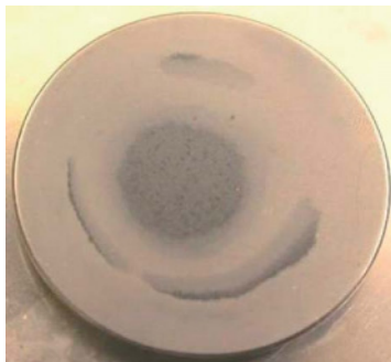
Fig. 2 Segregation structure of valve
