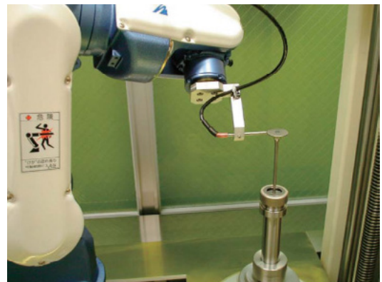
Fig. 4 Method of eddy current inspection
