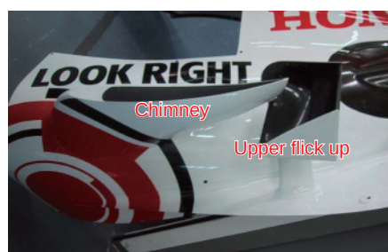
Fig. 28 Chimney and upper flick-up
