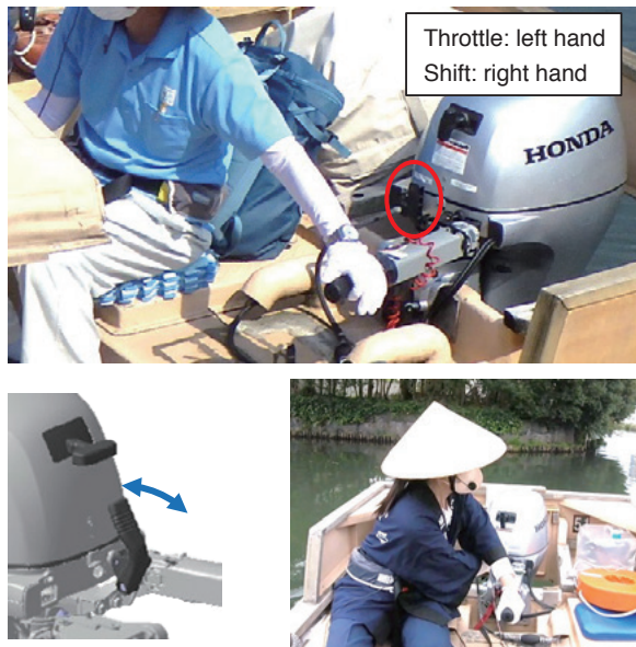
Fig. 10 Conventional method of shift switching
