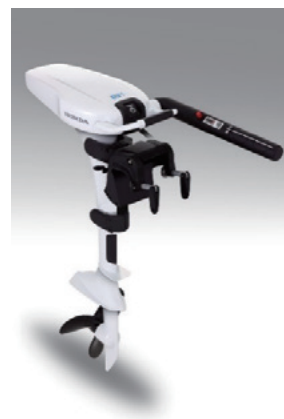
Fig. 1 Concept model of electric outboard motor for small boat
