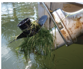
Fig. 17 Tangled algae around propeller
