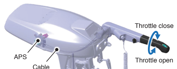
Fig. 13 APS position in electric outboard motor
