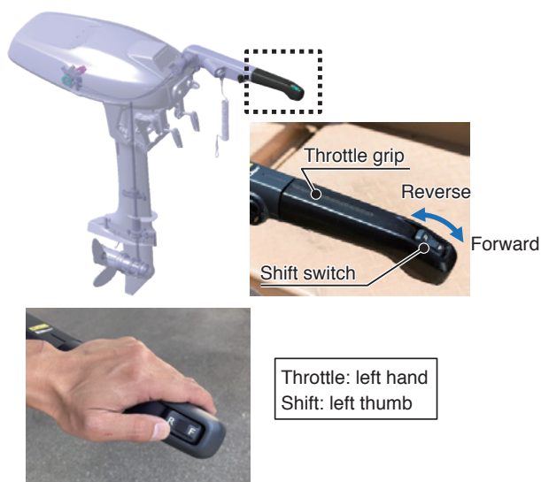
Fig. 11 New method of shifting by alternating switch
