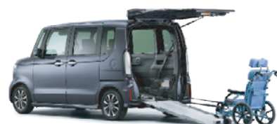
Fig. 2 Adapted vehicle with rear ramp
