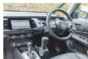
Fig. 1 Adapted vehicle with hand control device
