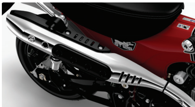
Fig. 24 Slim-looking muffler tucked along the frame
