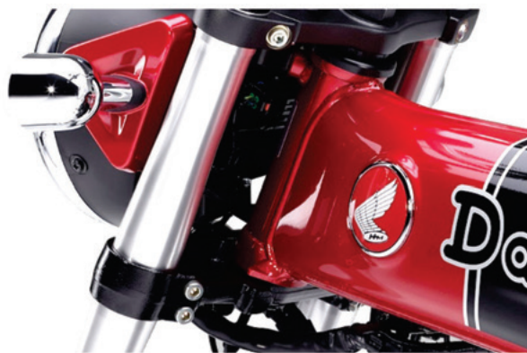
Fig. 21 Simple yet beautiful steering head pipe area without gusset
