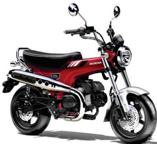
Fig. 13 Pressed steel frame having an optimum volume
