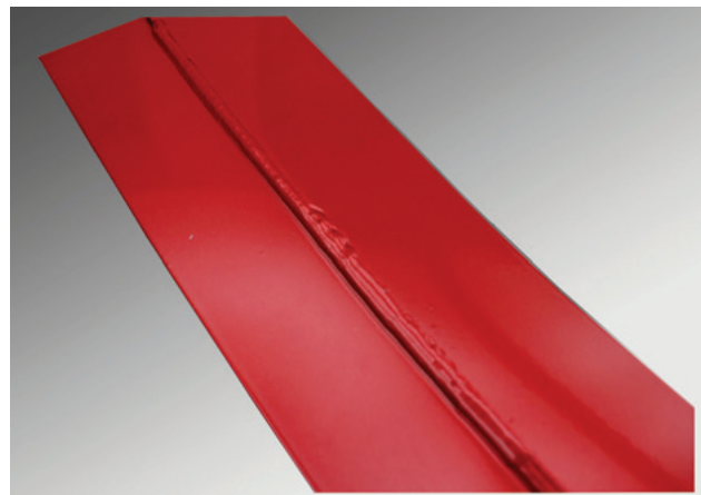
Fig. 19 Sample of welding bead appearance
