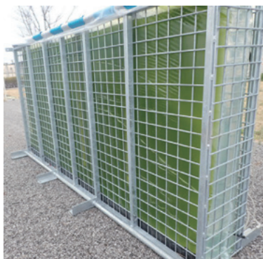
Fig. 18 Flat panel photobioreactors placed outdoors
