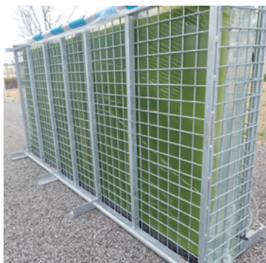
Fig. 18 Flat panel photobioreactors placed outdoors
