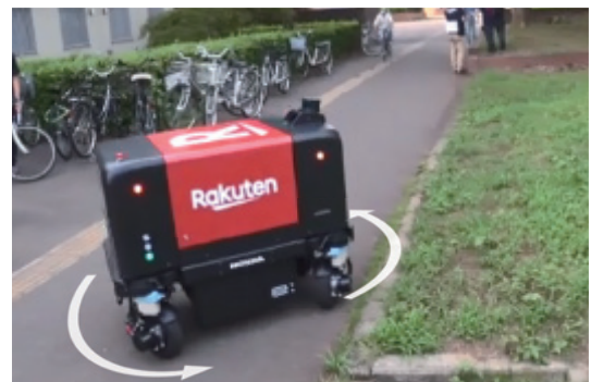
Fig. 19 Turning on spot on narrow road (Minimum turning radius: approximately 700 mm)
