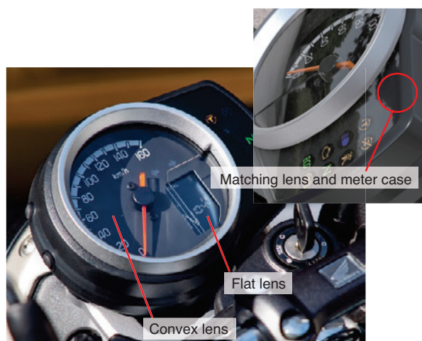
Fig. 20 Appearance of meter unit
