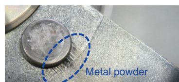
Fig. 11 Fretting abrasion on plane of rivet
