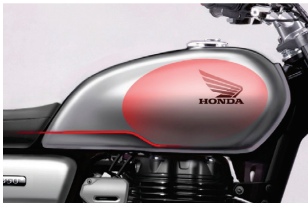
Fig. 14 Character line of fuel tank
