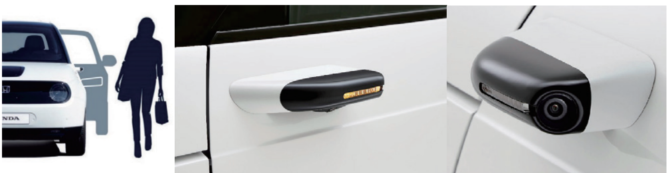
Fig. 9 Side camera mirror
