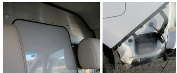
Fig. 8 Smoke leak test
