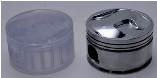
Fig. 13 Prototype produced by optical molding (left), prototype produced by metal 3D printer (right)
