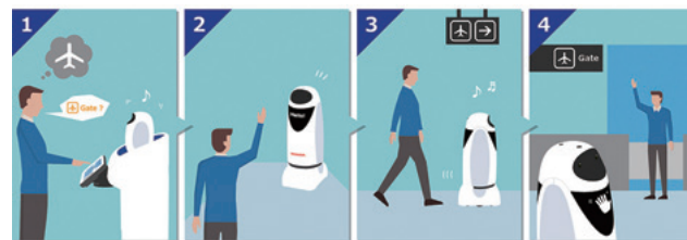
Fig. 3 Utilization flow of guide robot service
