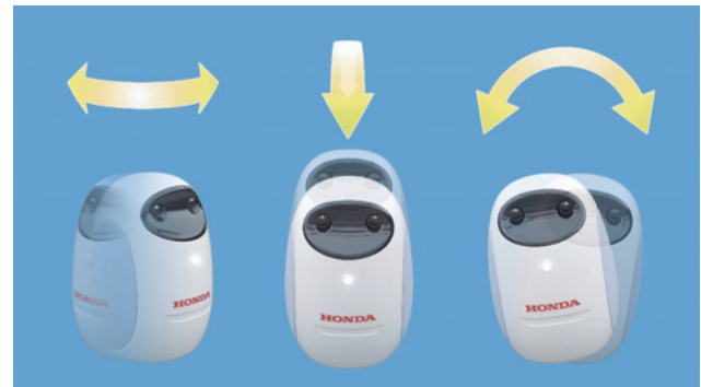
(a) Turning around (tracking person) (b) Bowing (receiving voice input) (c) Tilting (searching)
