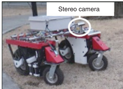
Fig. 6 Test robot with stereo camera
