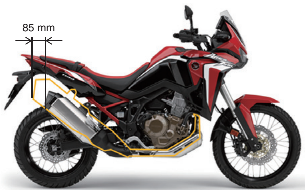
Fig. 11 Comparison of muffler size
