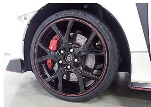
Fig. 17 Reverse rim wheel on sport type car
