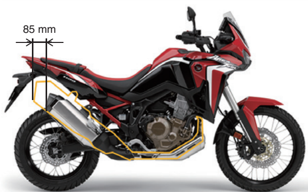
Fig. 11 Comparison of muffler size
