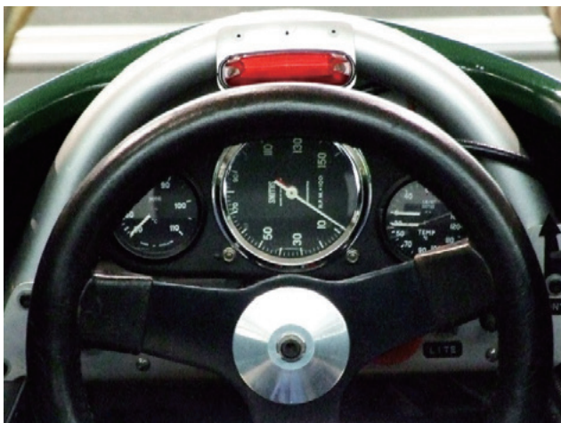
Fig. 5 Rotated tachometer on 1980 Ralt Honda racing car optimized to show upshifting of gears
