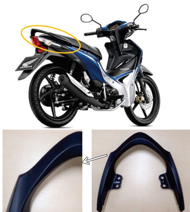
Fig. 25 Mass production rear grab rail of Heat and Cool molding applied to Thai model
