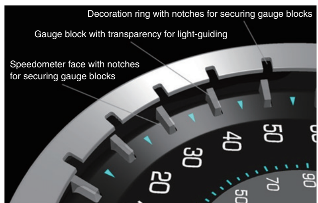
Fig. 21 Exploded view showing gauge ring construction
