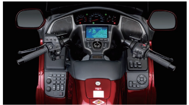
Fig. 3 Instrument cluster, handlebar switches, and body panels of previous model
