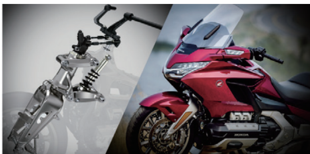
Fig. 16 Double wishbone type front suspension
