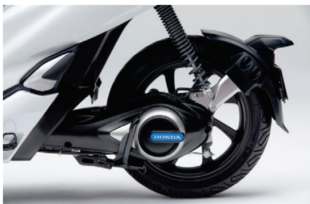
Fig. 31 External view of power unit
