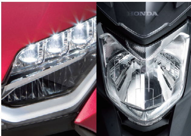
Fig. 9 Difference in appearance due to difference in structure of reflector
