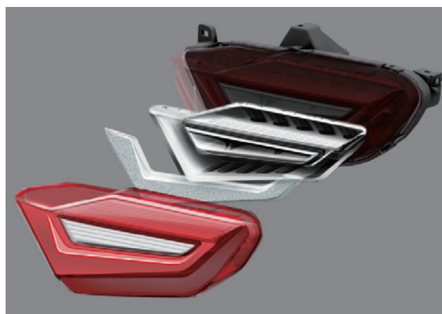
Fig. 15 Sketches of parts constructing combination light
