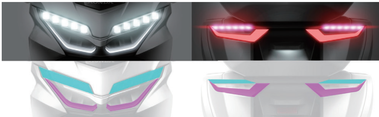
Fig. 14 Unified characteristic impression applied to front and rear lighting systems
