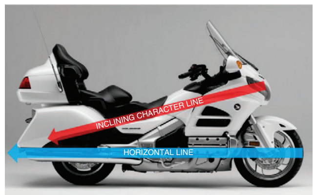
Fig. 7 Character lines applied to previous model of Gold Wing
