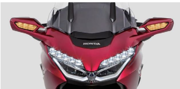
Fig. 17 Multi LED configured headlight adopting latest lighting technology for vehicles
