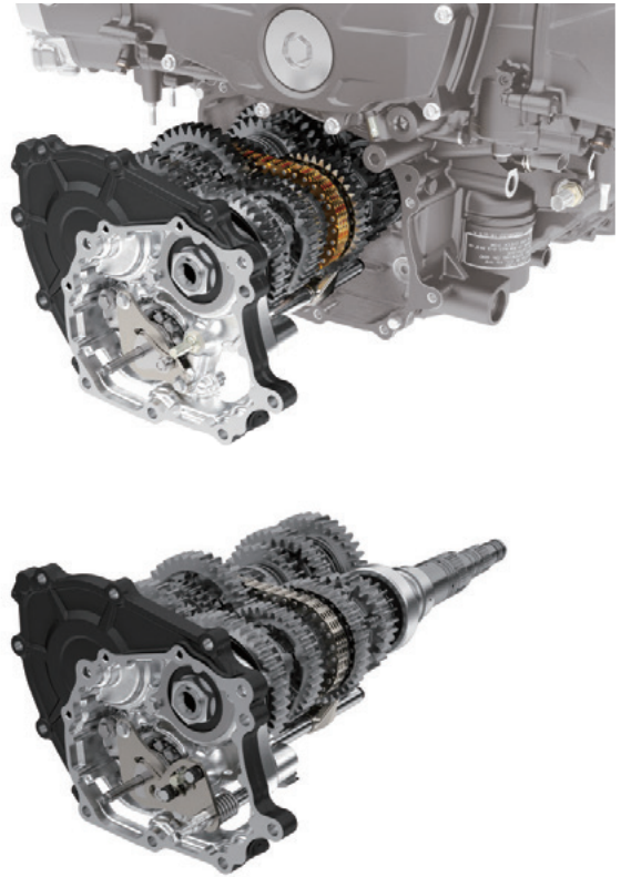
Fig. 4 Cassette transmission architecture
