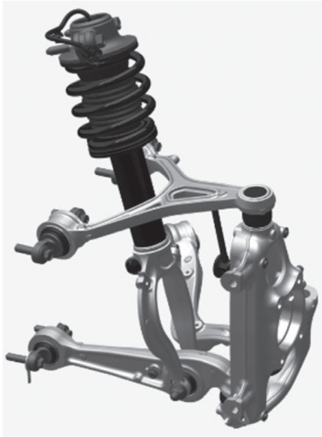
Fig. 2 Double wishbone type suspension for automobiles
