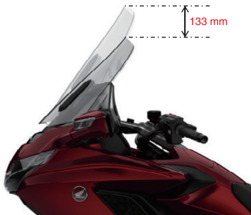
Fig. 26 External view of electronically controlled wind screen
