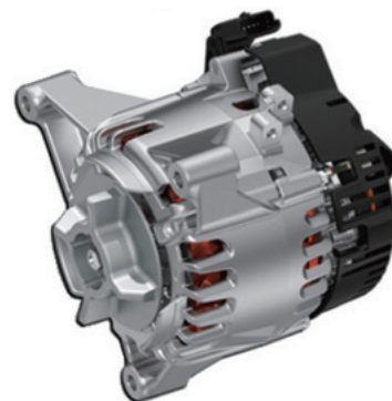
Fig. 9 Shape of ISG for developed Gold Wing
