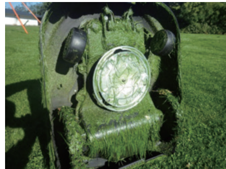
Fig. 10 Grass trimmings on mower underside
