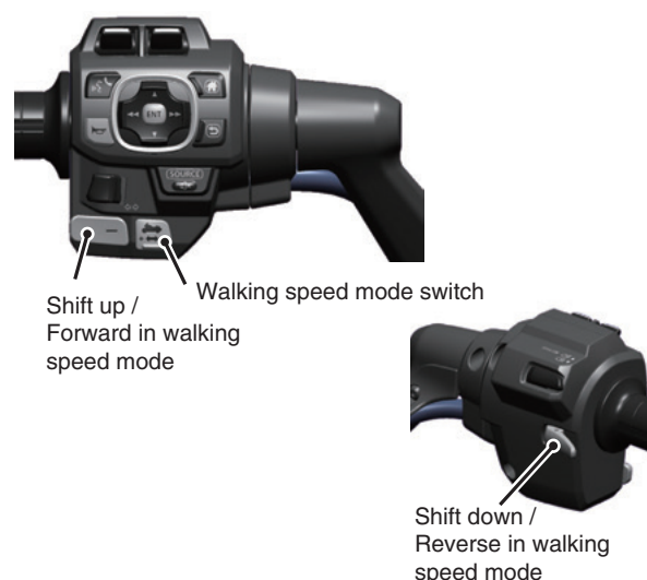
Fig. 5 View of left handle grip switches
