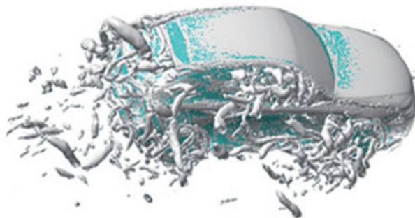
Fig. 4 Crosswind simulation image
