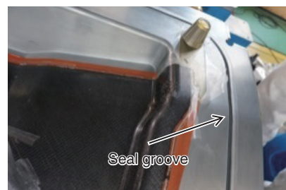
Fig. 14 Result for gap RTM mold after shot
