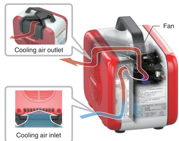
Fig. 14 Cooling air flow
