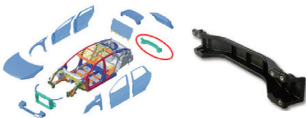
Fig. 9 Thermoplastic GFRP rear bumper beam and location in CLARITY FUEL CELL
