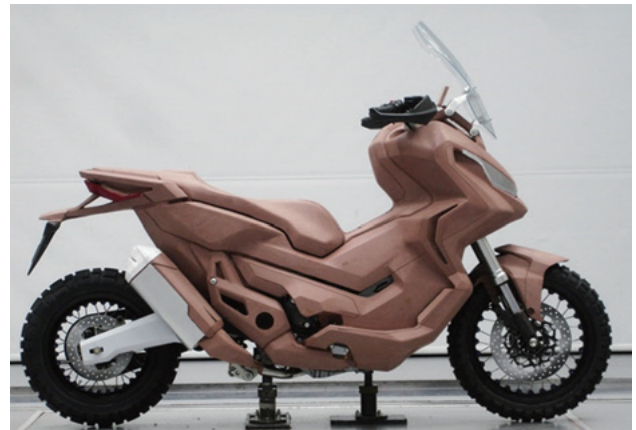
Fig. 11 Completed clay model
