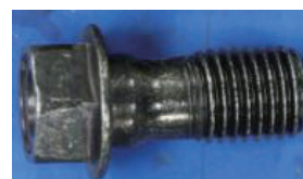
Appearance of coating bolts immersed in brake fluid after baking at 140^\circ C
