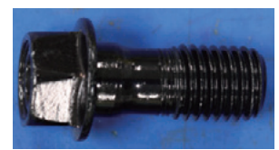
Appearance of coating bolts immersed in brake fluid after baking at 180^\circ C
