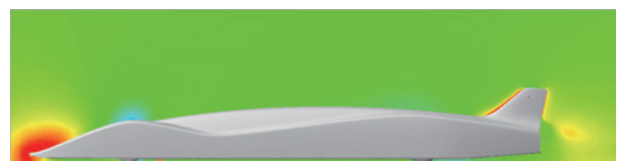
Fig. 12 Shape and section pressure distribution of race car model
