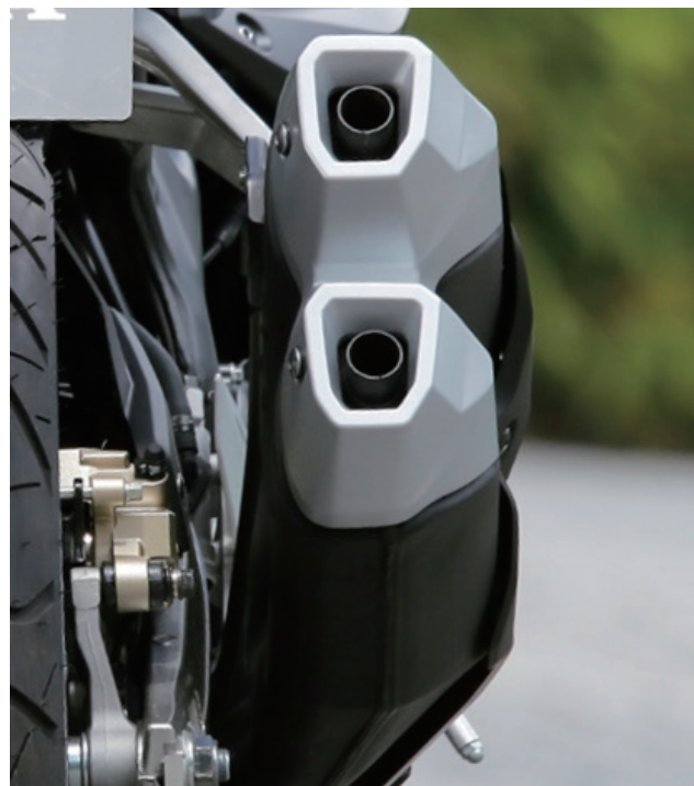
Fig. 35 Twin mufflers with variant cross sections
