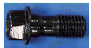
Appearance of coating bolts immersed in brake fluid after baking at 180^\circ C
