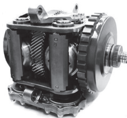
Fig. 3 Double-cavity half-toroidal variator
