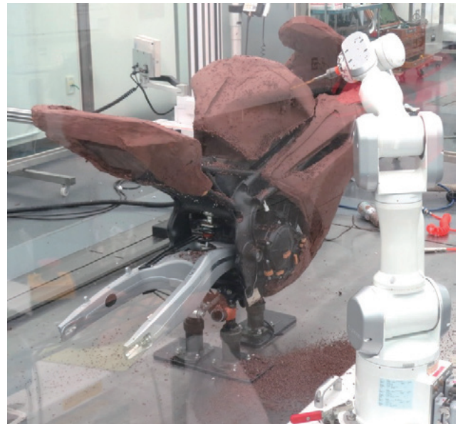
Fig. 22 Production of full scale clay model by numerically controlled clay trimmer
