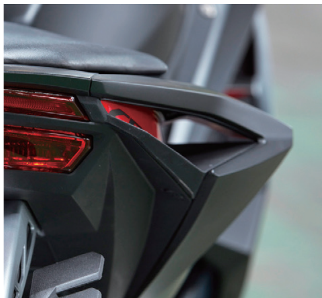
Fig. 33 Air outlets on rear cowl
