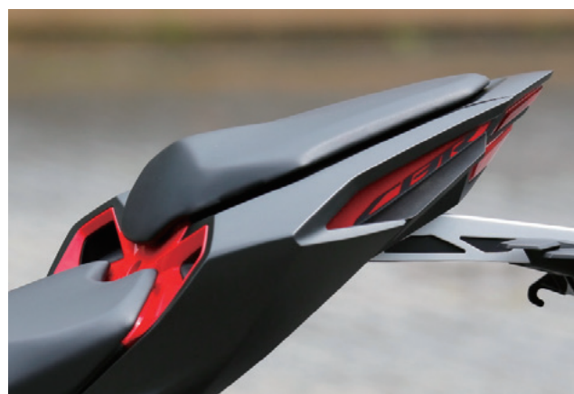
Fig. 34 Layered cowl and rear cowl expressing speed by wing shape
