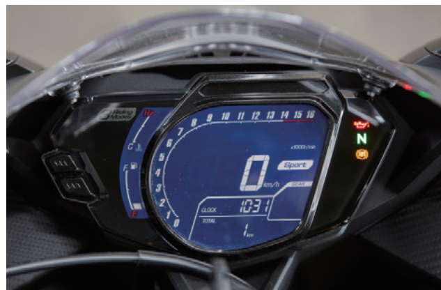
Fig. 36 Large-sized fully digitized gauge unit
