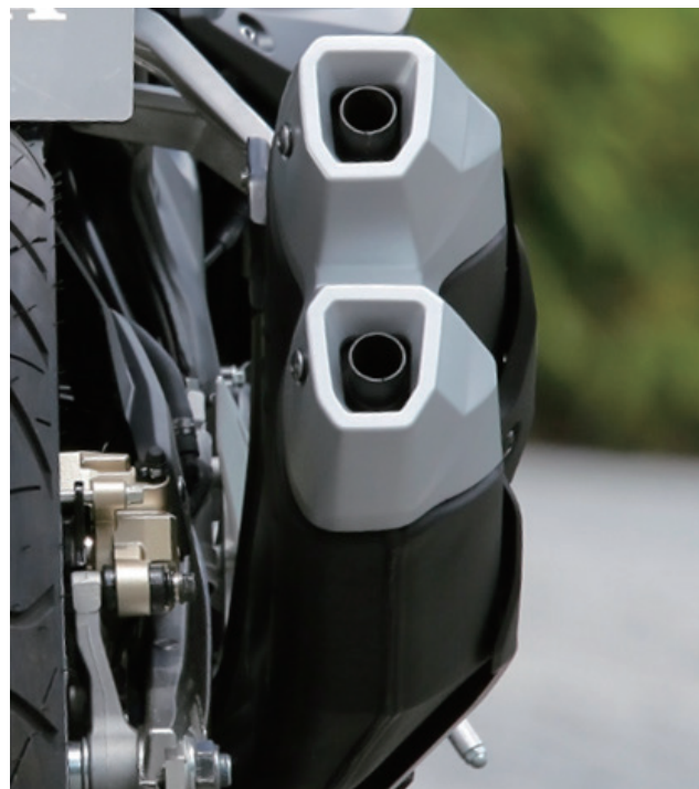
Fig. 35 Twin mufflers with variant cross sections
