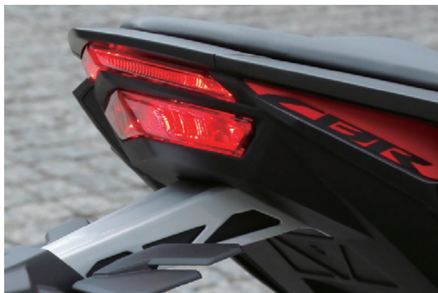
Fig. 31 Two tiered arrangement of upper and lower LED taillights
