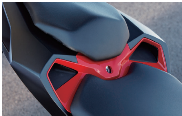
Fig. 32 Air guiding intake openings on rear cowl
