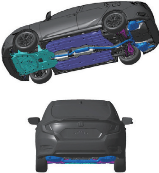
Fig. 8 Aerodynamic treatment on new CIVIC underfloor
