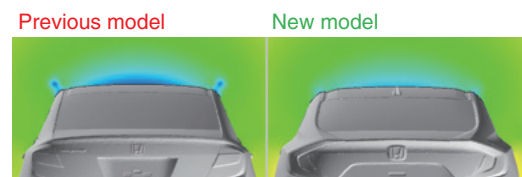
(b) Pressure difference between C-pillar and roof
