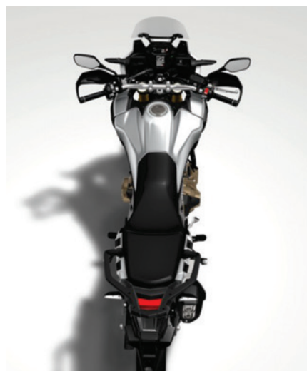
Fig. 13 Streamlined seat shape that helps smooth actions of a rider
