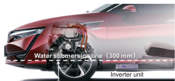
Fig. 21 Inverter mounting position
