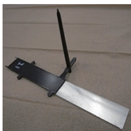
Fig. 9 Specimen of joined CF RTP and Al alloy
