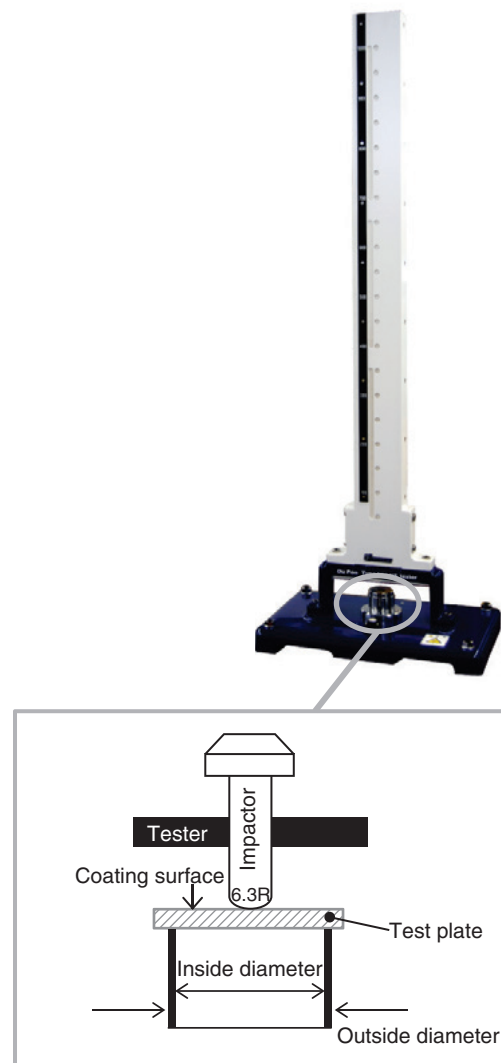
Fig. 4 Modified Dupont impact tester
