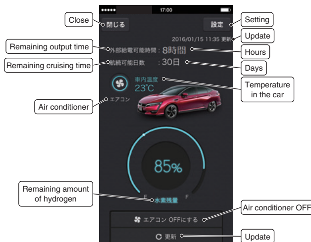
Fig. 15 Design example of internavi application on smartphone
