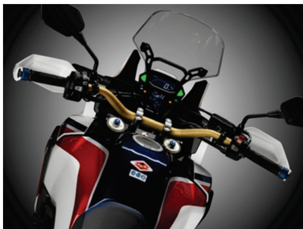
Fig. 20 Contrast in brightness by metallic colors applied to the painted areas and the stripes
