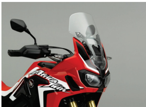
Fig. 14 Fairing with wind screen with a steep angle
