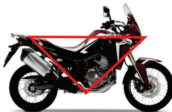
Fig. 12 V-shape proportional scheme applied to the new Africa Twin
