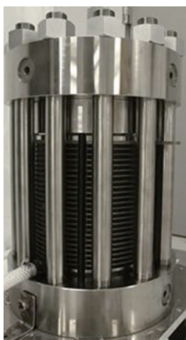
Fig. 12 Photograph of 70 MPa differential-pressure water electrolysis stack
